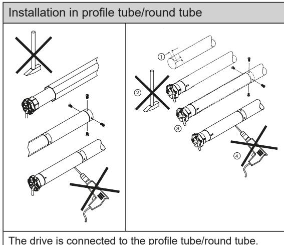
The drive is connected to the profile tube/round tube.
