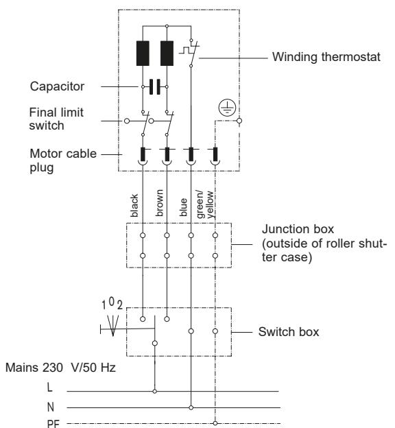
Fig. 4 Circuit diagram VariEco with 230 V / 50 Hz
