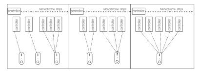
Caution: one controller can connect with up to four different remote;
