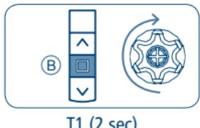
This first process brings the awning to the open position and sets the motor into "dead man" operating mode. Thereafter, the fabric tensioning position can be adjusted accurately.
