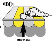
As long as the measured wind speed is higher than the adjusted threshold, any order is inhibited.
