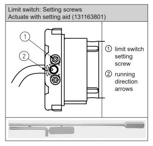
To actuate the limit switch setting screws, use the setting aid or a Phillips-tip or hexagon socket tool, but never a power screwdriver.
