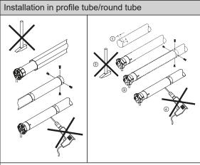
The drive is connected to the profile tube/round tube.
